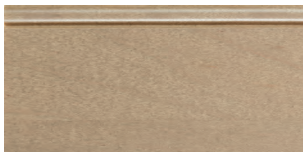
Fog stain on Maple
